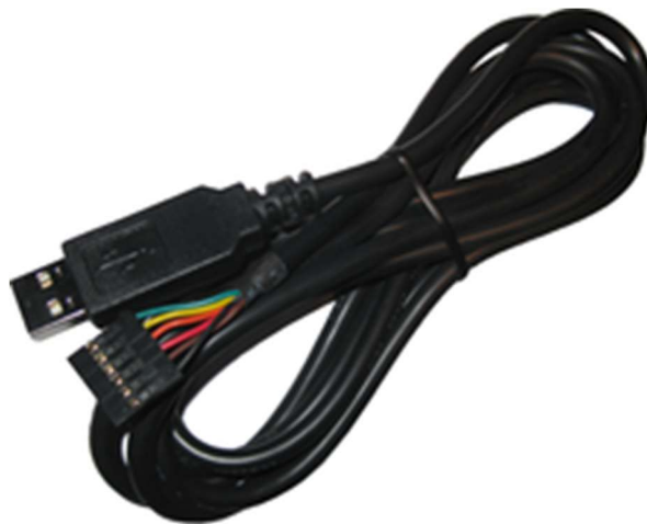
Figure 18: USB type A connector FTDI cable
